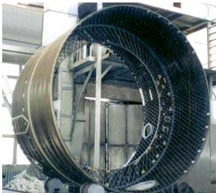
Fig.3. Equipment compartment of “Proton-M” LV Stage II
