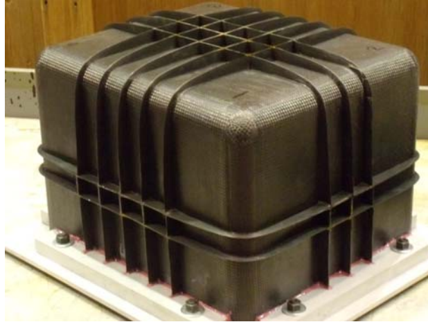
Figure 4: The final grid-stiffened composite pressure shroud
