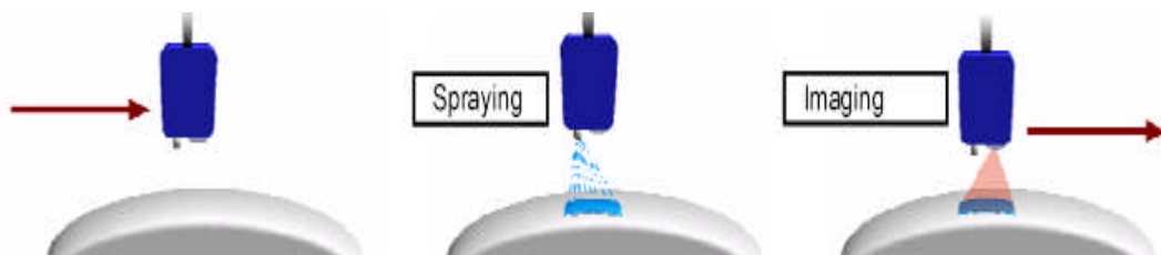
Fig. 10: Illustration of mobile aerosol wetting on curved FRP parts [7]
