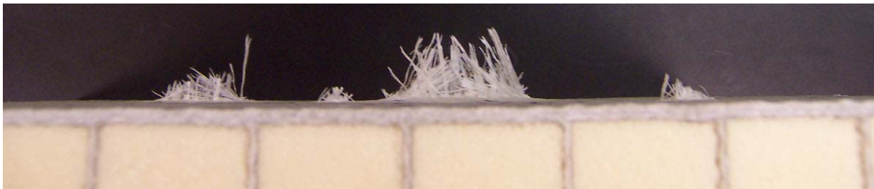
Figure 9. E-glass / Tycor vinyl ester sandwich – Side view (projectile exit)
