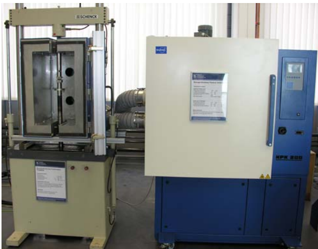
Fig. 6. Servo-hydraulic testing complex INSTRON PSB with climatic chamber
