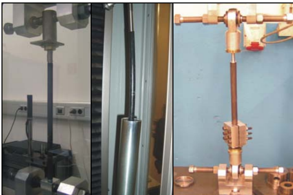
Fig. 9. C/SiC piston rods during structural testing
