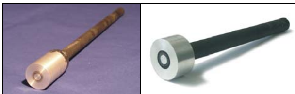
Fig. 12. CMC piston rods with cast-on aluminium (left) and magnesium working piston (right)
