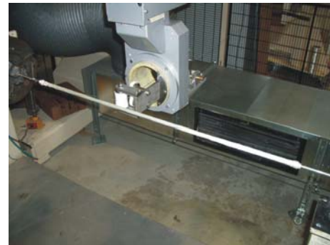
Fig. 3. Near-net-shaping of piston rod green bodies using filament winding
