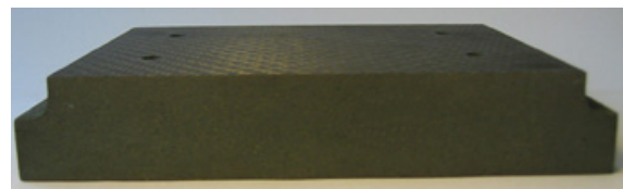
Fig. 24. Novel 3D textile reinforced CFC gliding element for maglev fabricated by Schunk
