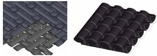
Fig. 2: Textile architecture of the investigated TTC (left: woven fabric, right: knitted fabric)
