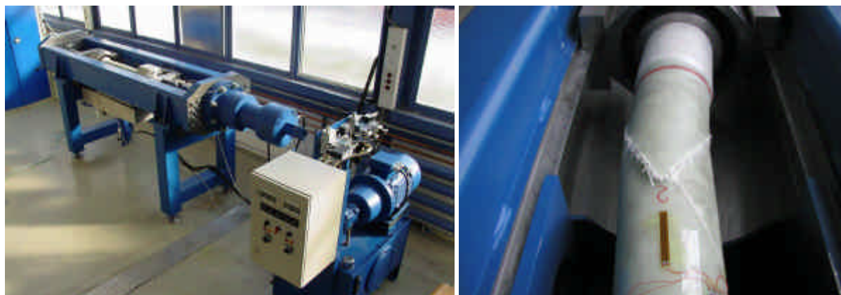
Fig. 17: Assembly of the pipe test stand for superimposed loading (T/C-p-b tests)
