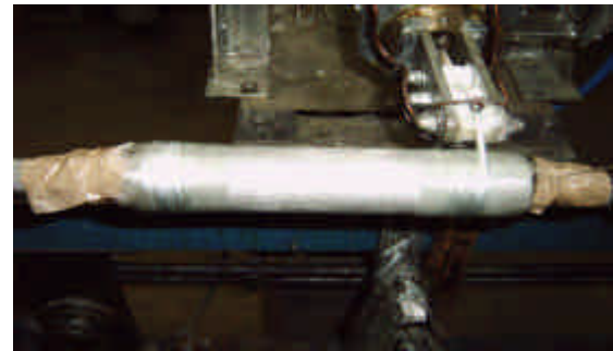
Fig. 7: Winding of the roving
