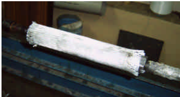
Fig. 6: Adding the weave pipe
