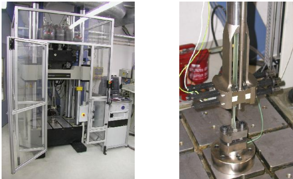
Fig. 1: Servo hydraulic high speed tension and penetration unit (SHU)
