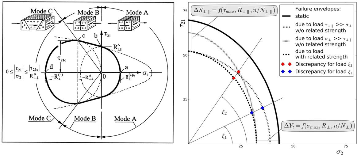
Figure 2:  $\sigma_2, \tau_{21}$  - failure envelope (also referred to as  $\sigma_{\perp}, \tau_{\perp\parallel}$  - envelope) for Puck's failure criterion [3] (left) and a schematic envelope with related and unrelated strength reduction in Mode A (right)
