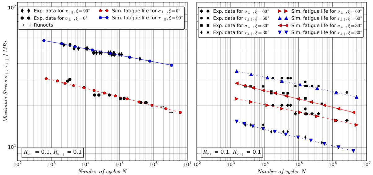
Figure 5: Verification for the average predicted life of input data  $\xi = 0^\circ$  and  $\xi = 90^\circ$  (Left) and Validation for  $\xi = 30^\circ$  and  $\xi = 60^\circ$  (Right)
