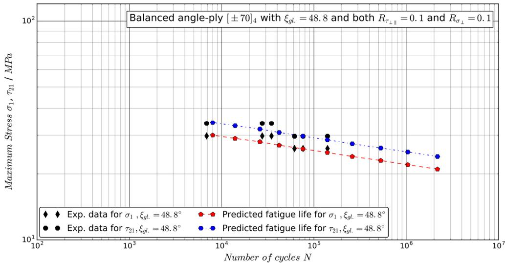
Figure 6: Balanced angle-ply tubes with stacking sequence  $[\pm 70]_4$  under biaxial loads with a global biaxiality angle of  $\xi_{gl.} = 48.8^\circ$  and proportional stress ratios  $R_{\perp\parallel} = R_{\perp} = 0.1$ .
