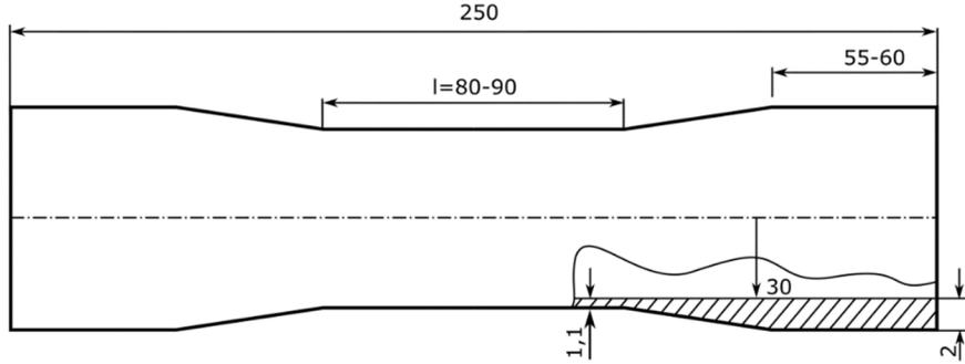
Figure 3: Geometry of CFRP-specimen for combined tension-torsion loads
