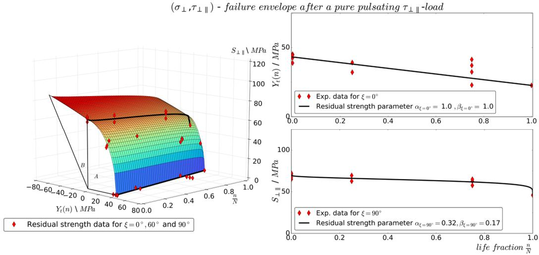
Figure 4: Homothetic failure envelope after a pure pulsating in-plane shear load with stress ratio  $R=0.1$  (left) and the estimation of the residual strength parameters with residual strength data for  $\tau_{\perp\parallel}$  and  $\sigma_{\perp}$  after 25% and 75% of fatigue life (right).
