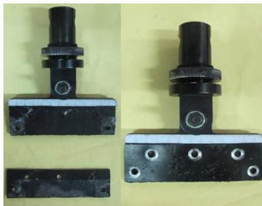
Figure 1: The grips used in bias extension test.
