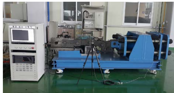
Fig. 2 Long pitch roller chain wear test machine
