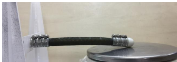
Figure 4: Block Force Test: One end of actuator clamped on the test frame, and the other contacting with the force sensor
