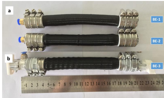
Figure 1: The Bending Extensile PAM composed of two end fittings, an elastic tube, a braid tube and an embedded elastic frame.
