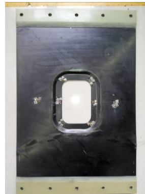
Figure 1: The damage zone of the flanging configuration plate
