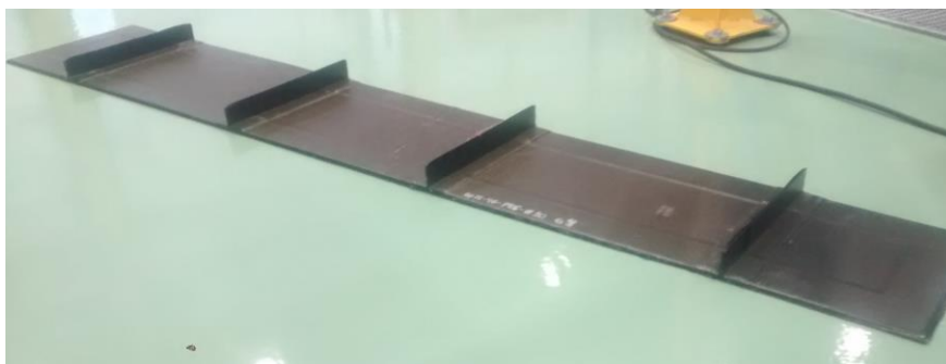
Figure. 1 Front Spar cured using DVD technique
