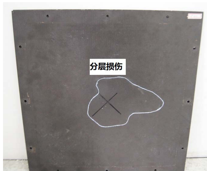
Figure 3: Impact damage in the CFRP laminate caused by high velocity hail impact
