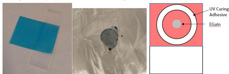
Fig. 2: ITO coated PET with transparent tape mask (left), deposited layer of PEDOT:PSS (center), Layout for EGaln and UV adhesive (right)
