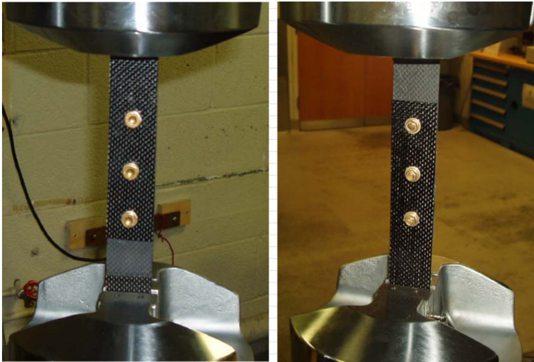
Figure 1 Front and back faces of a 3-Bolts specimen mounted on MTS 810 Machine
