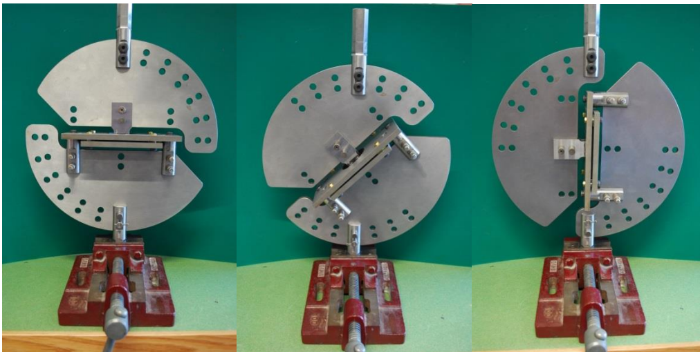
Figure 7: Novel ARCAN bolted joint fixture pictured in pull-through (left), combined loading (centre) and bearing (right) configurations
