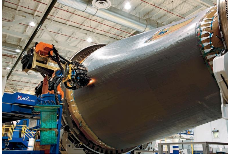
Figure 1: Example of automated material placement technology employed in production of composite components for commercial airliners (reproduced from Lewis [1]).
