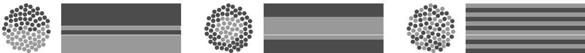
Figure 1: Variations of hybrid yarns (after [2]); left: side by side, middle: core skin, right: mixed
