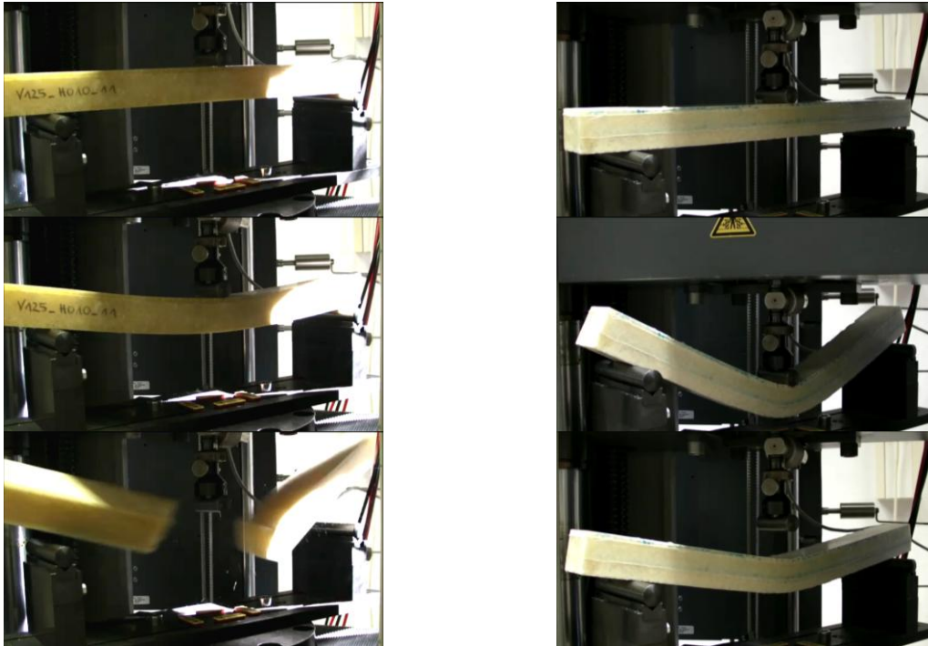
Figure 3: Process of the bending test according to DIN EN ISO 178 (snapshots) of a reference foam sample (left) and a composite specimen of the SF2 series in two layers (right) [5]
