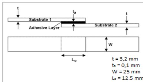
Figure 2. Geometry of specimens (mm)
