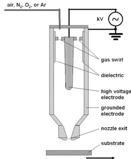
Figure 1. Components of an atmospheric pressure plasma torch
