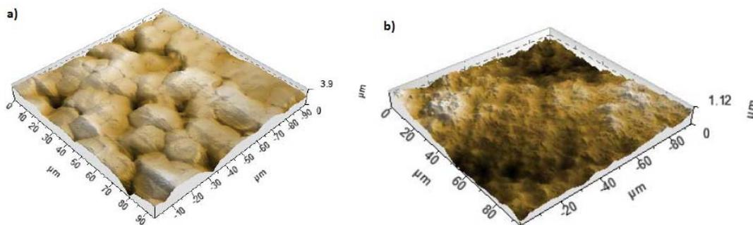
Figure 3. AFM 3D topographic images of polypropylene composite surface subjected to atmospheric plasma treatment with different operational parameter combinations (nozzle-to-sample distance/treatment rate), (a) plasma parameters reference PS1: h, v; (b) plasma parameters reference PS2: 2h, 2v
