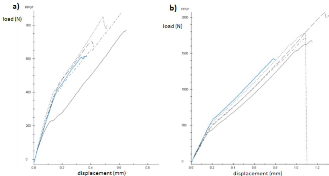
Figure 4. Lap shear test results of five specimens tested for both combinations of operational parameters; a) treatment referenced as PS1 (h, v), b) treatment referenced as PS2 (2h, 2v)
