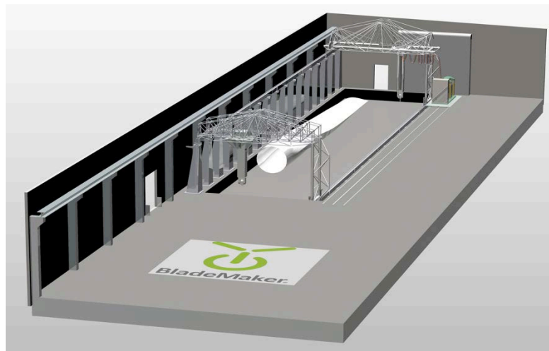
Figure 3: BladeMaker Demo Center for the industrialized production of rotor blades equipped with a flexible CNC-controlled gantry system, blade molds, mixing units etc.
