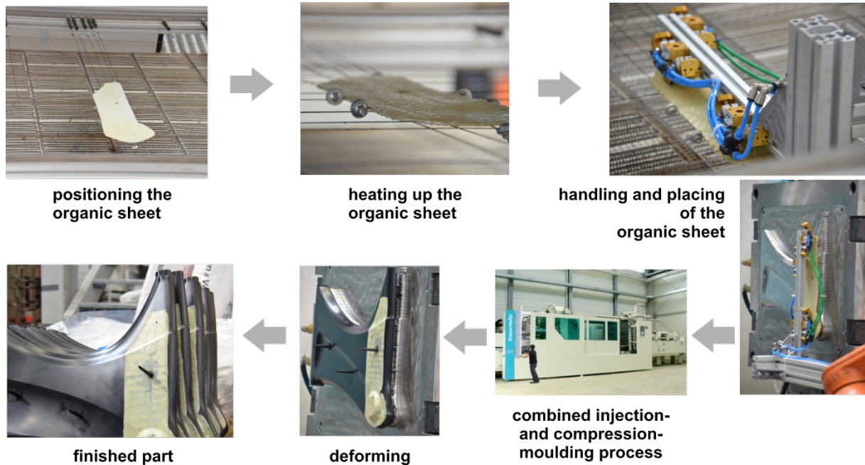
Figure 3: Steps of the manufacturing process
