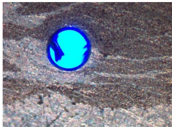
Figure 11: Test of the blue light transfer through Quartz UV 300/330 BN without coating using a stereoscopic microscope.
