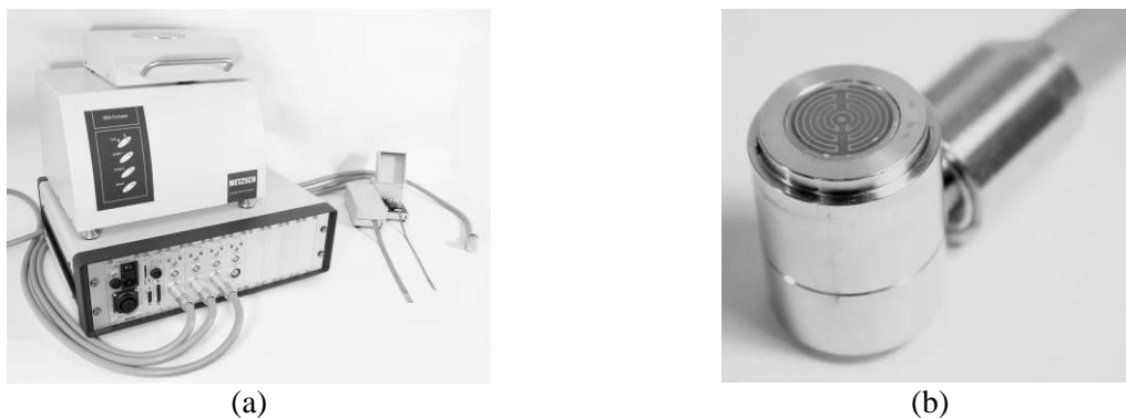
Figure 2: (a) Netzsch DEA288 and (b) tool-mountable sensor.
