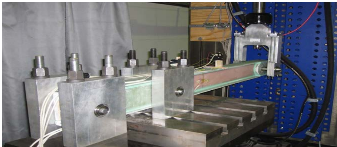
Figure 5: test set-up for a subcomponent test of a bond line between shear web and spar cap.
