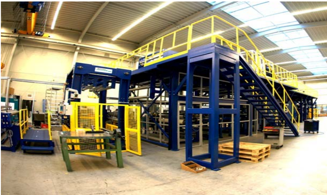
Figure 8. Production line: 1–10 m/min - Roller width 2.200 mm - Working width 2.000 mm
