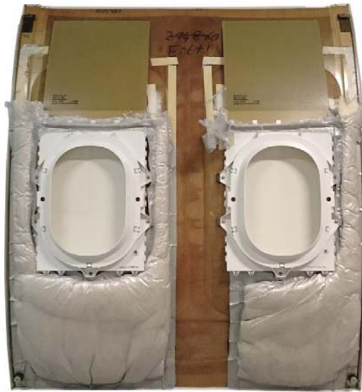
Figure 5. Sidewall-panel of an Airbus A320 from the backside. Photo: Fraunhofer PYCO.
