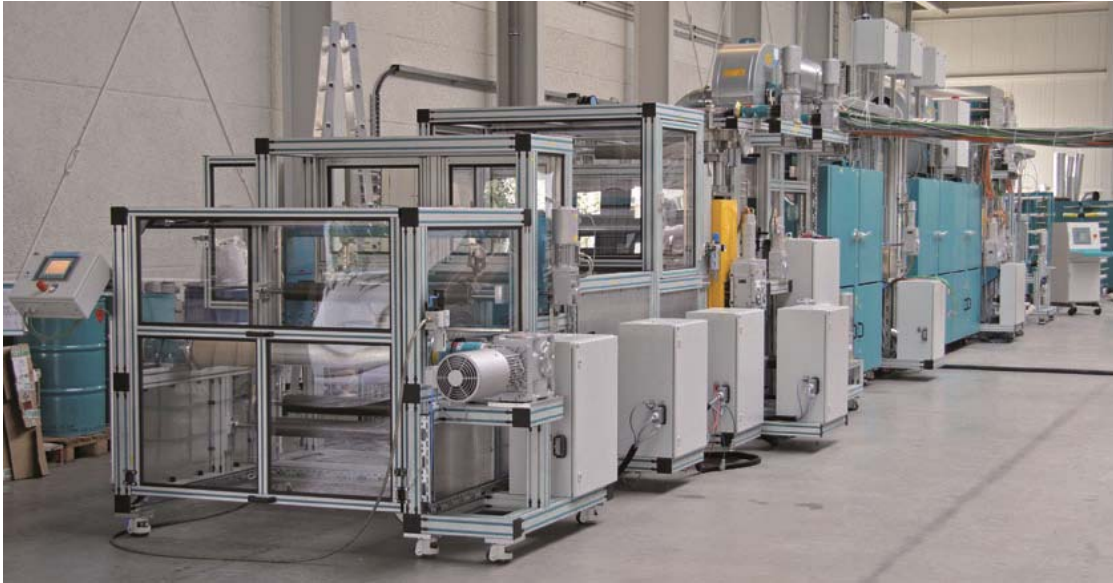
Figure 7. Lab Line: 0,1–20 m/min - Roller width 1.000 mm - Working width 800 mm
