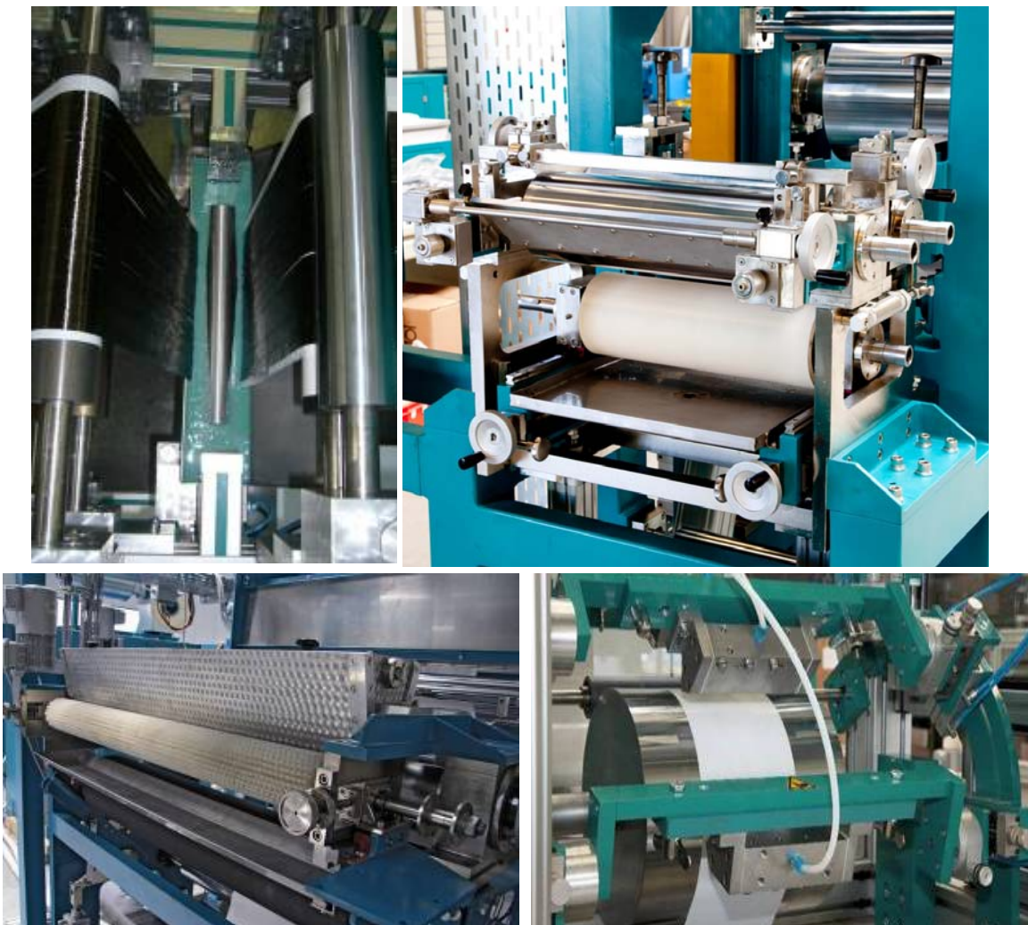
Figure 6. Typical coating technologies: Foulard, 3 Roller, Powder Scattering, Slot die. Photo: Coatema.
