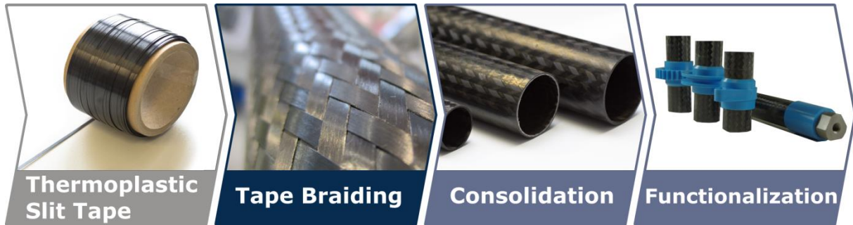
Figure 1: Manufacturing process for tape based FRT profile structures [1]
