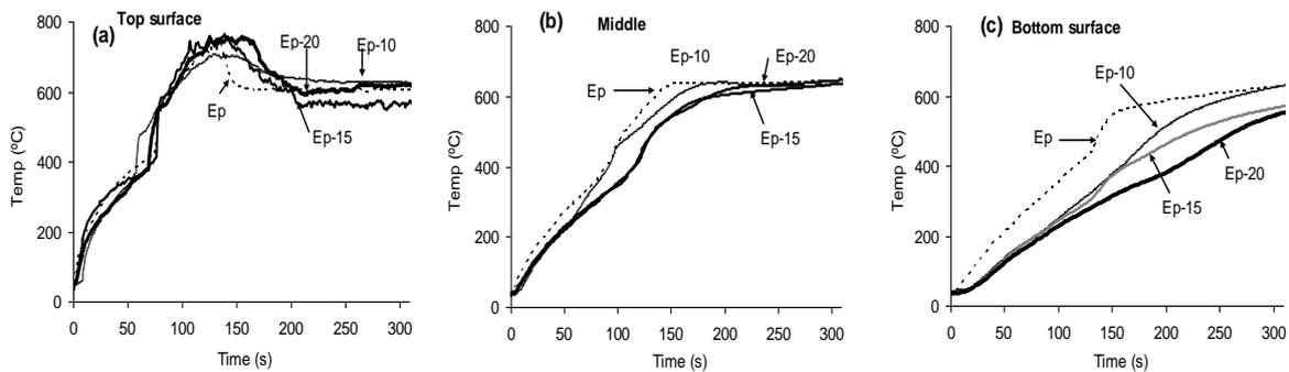
Figure 4. Temperature profiles in of composites at a) the exposed, b) middle and c) unheated surfaces of epoxy composites exposed to an incident heat flux of  $50 \text{ kW/m}^2$ .
