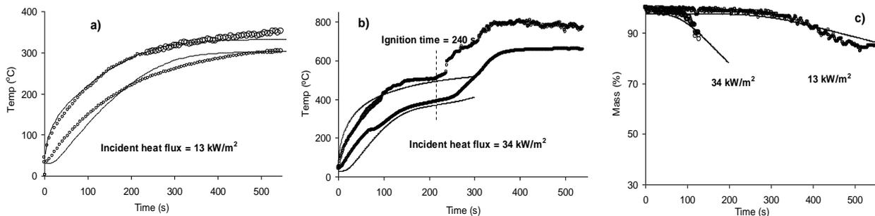
Figure 5. Experimental (data points) and predicted (solid lines) temperature profiles and mass loss data for control epoxy composite.
