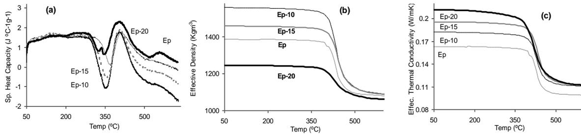
Figure 2. a) Specific heat capacity, b) effective density and c) effective thermal conductivity of different composites as a function of temperature.
