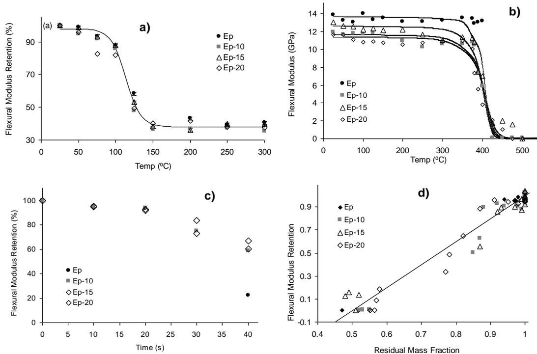
Figure 7: Residual flexural modulus retention of composites as measured a) at elevated temperatures, b) after exposure to elevated temperatures followed by rapid cooling to ambient temperature, c) after exposure to a 50 kW/m<sup>2</sup> heat flux, and d) flexural modulus retention after exposure to elevated temperatures followed by rapid cooling to ambient temperature versus the residual mass fraction.
