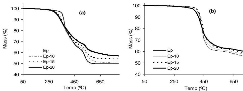
Figure 1. TGA curves of composites at 10 and 200 °C/min in flowing air
