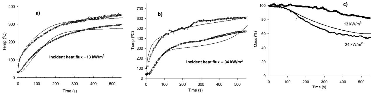
Figure 6. Experimental (data points) and predicted (solid lines) temperature profiles and mass loss data for Ep-20 composite.
