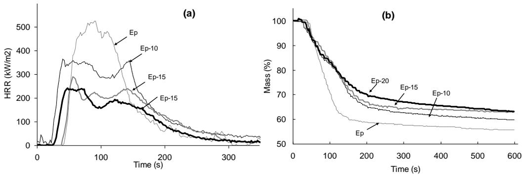
Figure 3: (a) Heat release rate and (b) mass loss curves as a function of time for composites from cone calorimetry measurements at  $50 \text{ kW/m}^2$ .
