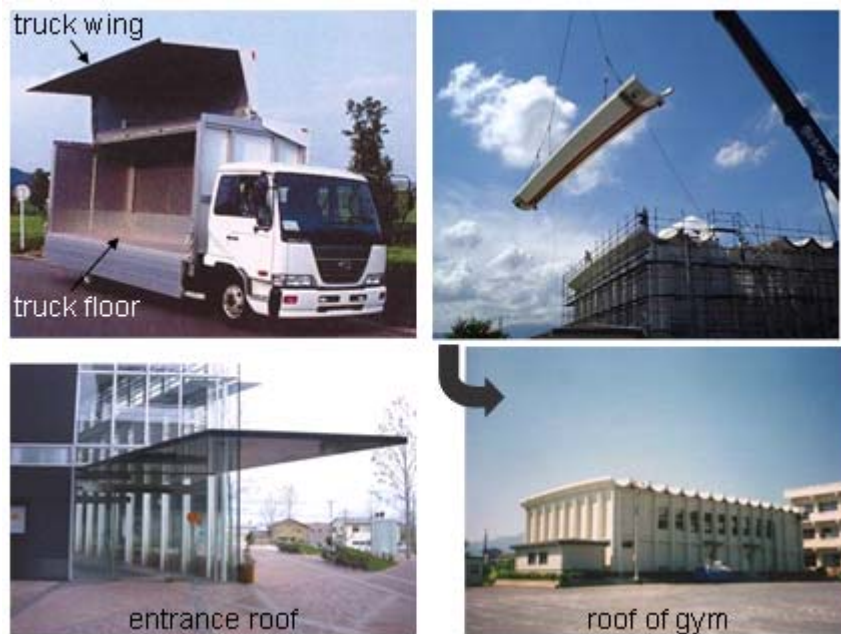
Figure 2 Examples of applications of VaRTM process
