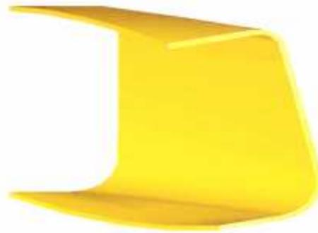
Fig 12. magnified spring-in geometries for a relatively long “C” section
