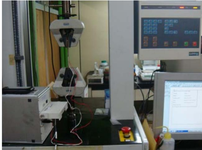
Fig.8 Tensile and strain gauge test
