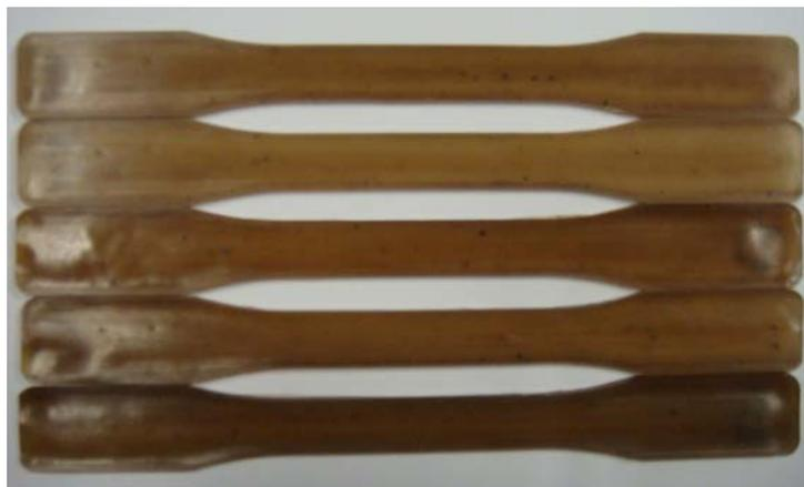
Fig.7 7wt% nanoclay reinforced PP specimens for mechanical tensile test
