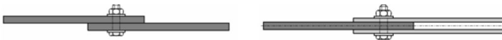
Fig. 5 - Schematic representation of single-bolt single lap joint and single-bolt double lap joint tests [16]
