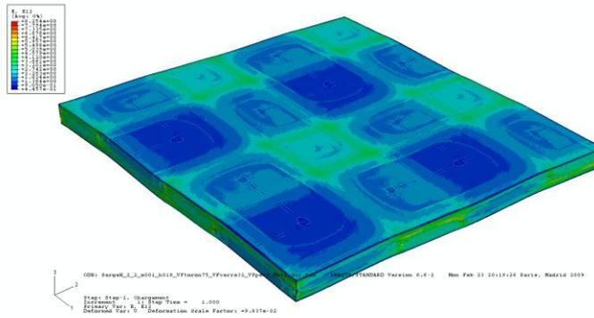
Figure 4: Hybrid twill weave on a shear loading in the plane
