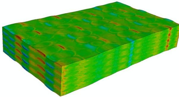
*Figure 6: Unbalanced layer/layer interlock out-of-plane shear on a tensile loading.*
