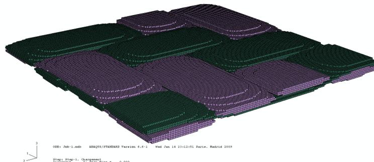
*Figure 3 : Example of a twill weave Glass/Vinylester coarse-meshed through the Voxel technique (1 M of DOF)*
