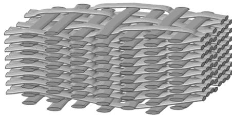
Figure 2: Representation of a complex 3D interlock woven fabric composite
