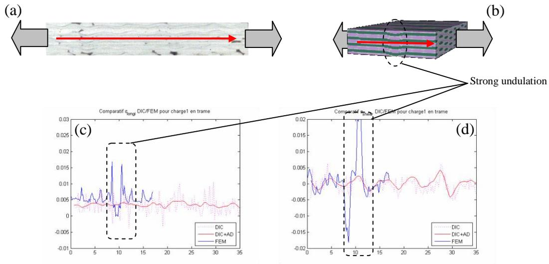
Fig. 7 Comparison of measured and computed longitudinal strain (c) and shear strain(d) along lines defined in the real woven (a) and the modelling (b)
