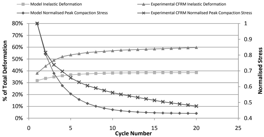
Figure 2: Multiple Cycle Compaction - Inelastic Deformation following each cycle and Normalised Peak Compaction Stress vs. Cycle Number
