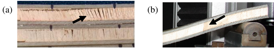
Figure 7 : Failure mode observed in (a) Parent :180 span (b)Parent:460 span
