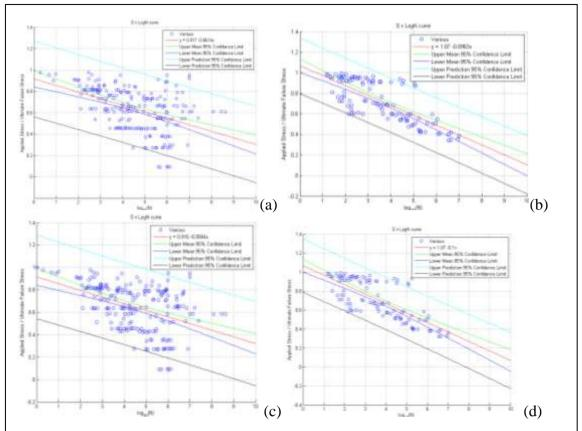
Figure 1: Graphs showing fatigue data of carbon fibre composites in compression and tension (a) and bending (b) and the data after the application of the Rotem model for compression and tension (c) and bending (d)
