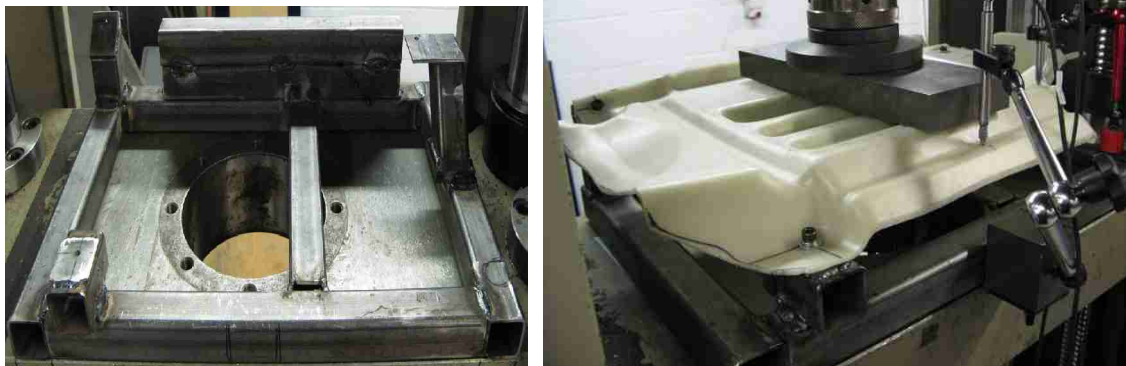
Figure 2 Frame for holding the foot-well panel
