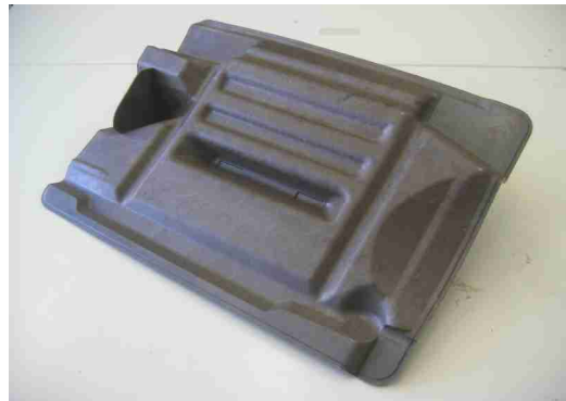
Figure 1 Flax/PLA interior floor-well panel.
