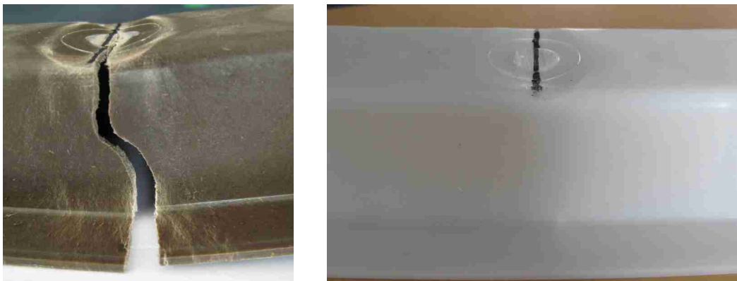
Figure 8 Failure modes of the flax/PLA and glass filled/polypropylene beams
