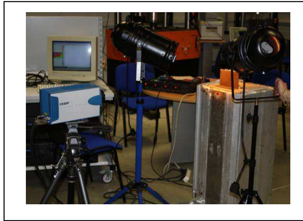
Figure 5: Thermography IR device.
