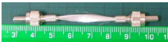
Figure 1 Photograph of an E-fibre bundle with a pair of polished SMA connectors.
