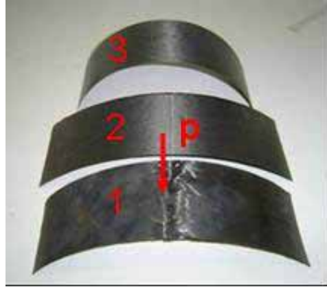
Fig.2 Three bistable laminates with different materials ply.
