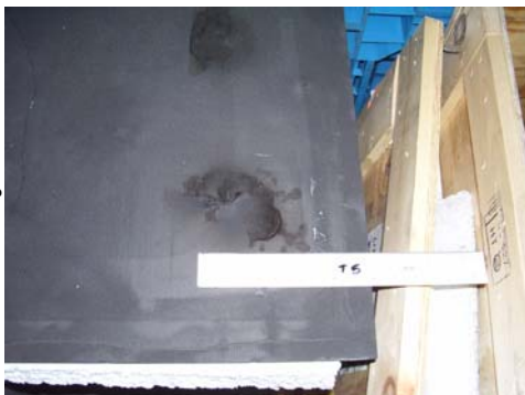
Figure 10: CARBON FOAM AFTER 100000 AMP LIGHTNING G STRIKE
