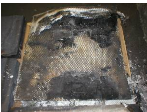
Figure 5: 7.5CM BALS PANEL DESTROYED IN FIRE
