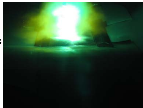
Figure 9: CARBON FOAM DURING 200000 AMP LIGHTNING STRIKE
