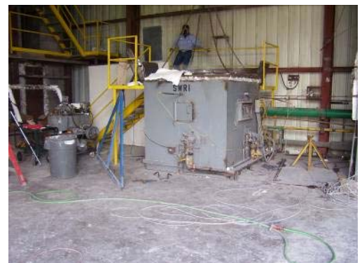
Figure 7: SWRI HORIZONTAL FIRE TEST FURNACE
