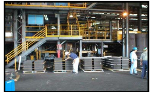
Figure 1: LARGE SCALE PRODUCTION OF GRAFOAM ® PANELS
