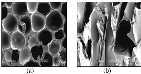
Fig. 1. SEM micrographs illustrating (a) as-cast neat PUR foam sonicated at 50A-30M (b) neat PUR foam sonicated at 50A-30M post static compression testing.
