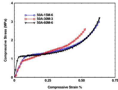
Fig. 2. Static Compression Test – Stress vs. Strain curve for 50A PUR foam.
