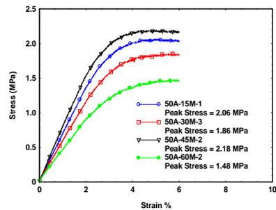
Fig. 3. Flexural Test – Stress vs. Strain curve for 50A PUR foam.
