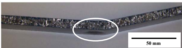
Fig.17. Failure in the damaged zone for thicker samples and larger damaged zones if the damaged zone is in a tensile loading condition.
