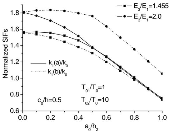
Fig. 5. Influences of the crack length and modulus ratio on the normalized TSIFs for an embedded crack in a 3-layered structure
