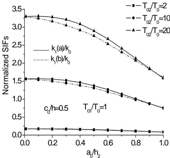
Fig. 4. Influences of the crack length and temperature variations on the normalized TSIFs for an embedded crack in a 3-layered structure
