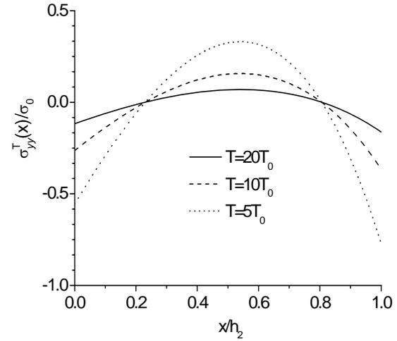
Fig. 2. Normalized thermal stress distribution in a (Rene-41)/Zirconia FGM layer
