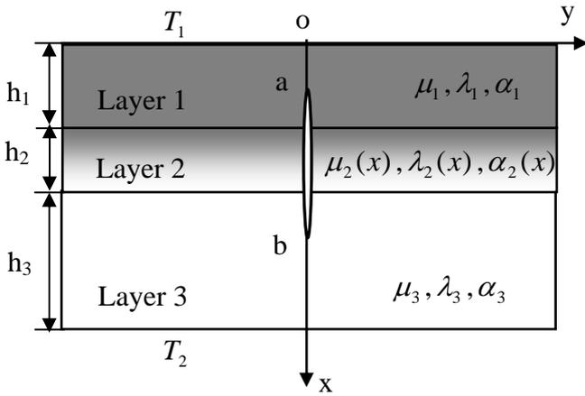
Fig. 1. Functionally graded layered structure with a crack intersecting the interface
