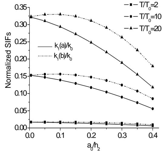
Fig. 3. Normalized TSIFs for an embedded crack in a (Rene-41)/Zirconia FGM layer
