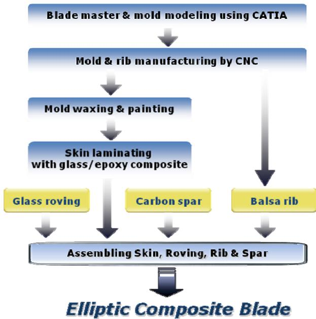
Fig. 13. Blade manufacturing process
