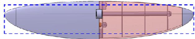
Fig. 3. Planform of the blade
