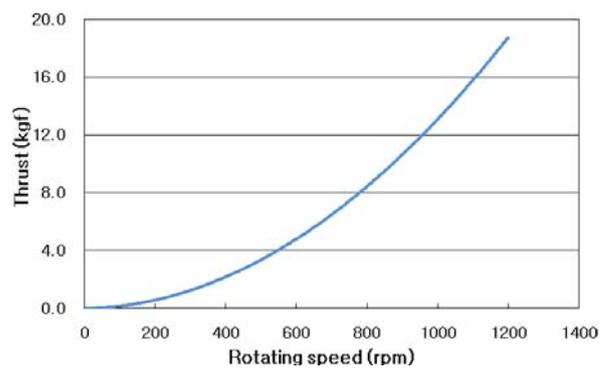
Fig. 4. Thrust variation according to rotating speed
