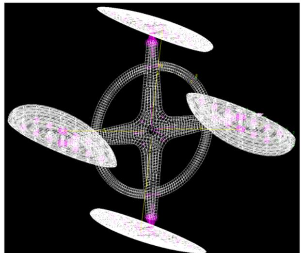
Fig. 8. FE mesh of cyclocopter rotor
