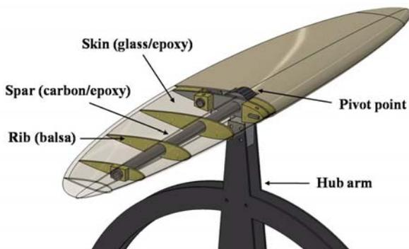
Fig. 7. Assembled picture of rotor blade
