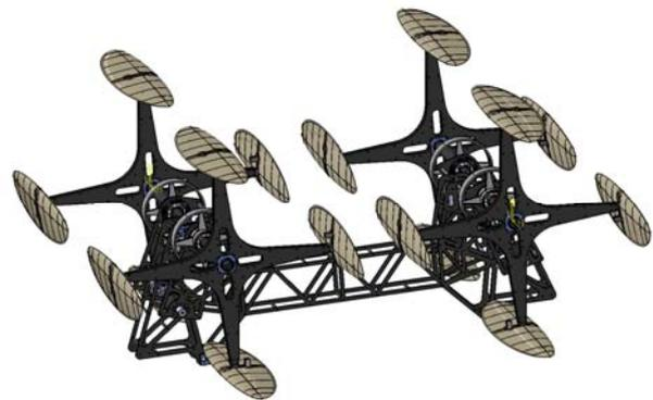
Fig. 1. Designed cyclocopter
