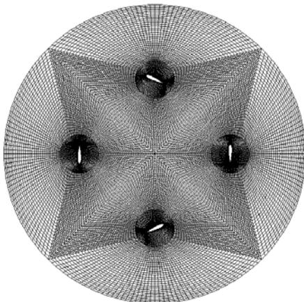
Fig. 2. Generated 2D mesh around the rotor
