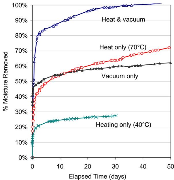
Fig. 5 Effect of temperature and vacuum
