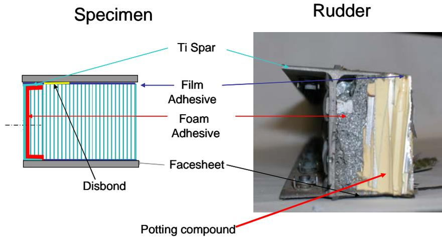
Fig. 3: Cross-section of leading edge of CF-18 rudder (left: design schematic, right: actual specimen)
