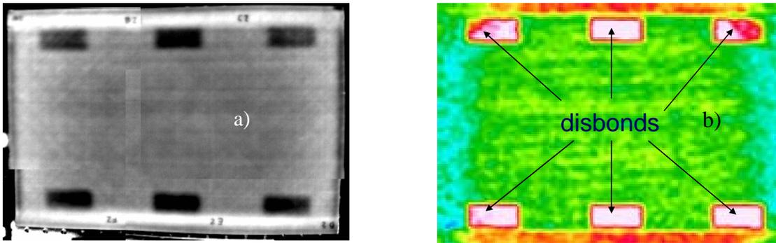
Fig. 4: NDI inspection of the fabricated sandwich panels (460mm X 280mm) with removed adhesive in six simulated disbonded areas of 25mm X 50 mm using a) Thermography b) Ultrasonic Inspection
