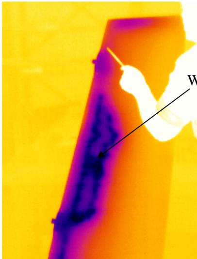
Fig. 9 Thermography image showing moisture ingress area in a CF18 rudder panel
