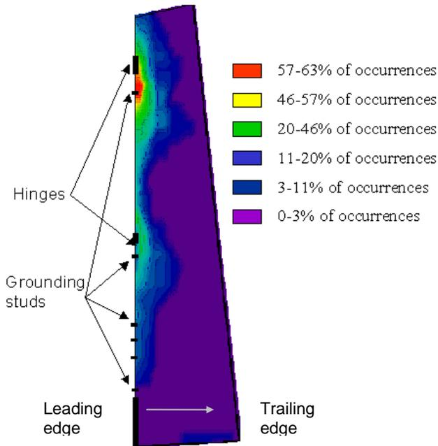
Fig. 2 Water ingress cumulative occurrence map developed based on 202 CF-18 rudders inspected between 1999-2004 using thermography.
