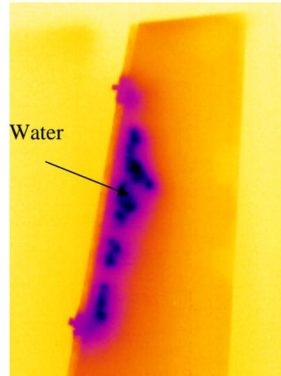
Fig. 11 Moisture ingress area after 8 hours of vacuum-assisted drying at 70 °C
