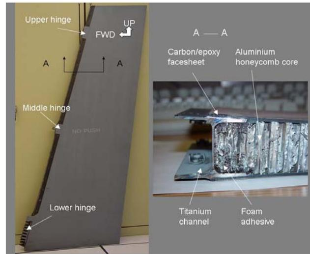
Fig. 1 Configuration of CF-18 rudder
