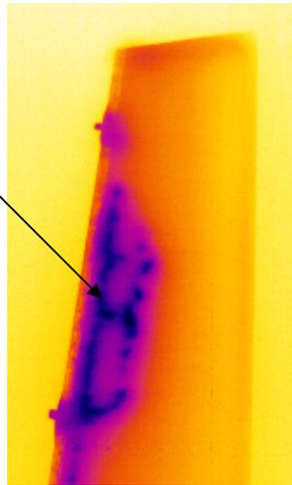
Fig. 10 Moisture ingress area after two months of moisture removal at around 80 °C
