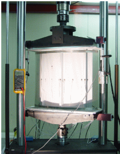
Fig. 1. Compressive load apparatus for buckling test
